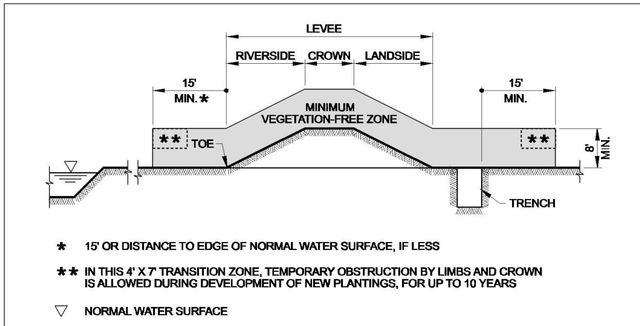
Figure A-6. Levee Section with Pervious Toe Trench.
